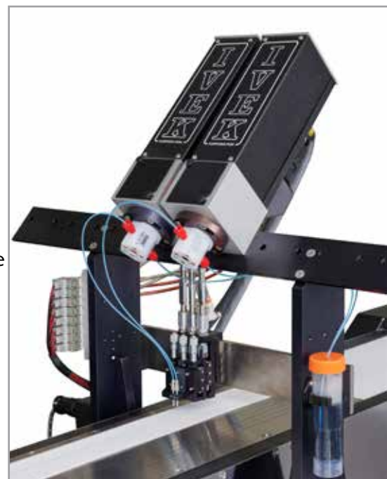
Linear Reagent Striper with 2 Linear Actuators mounted (2-tips)
